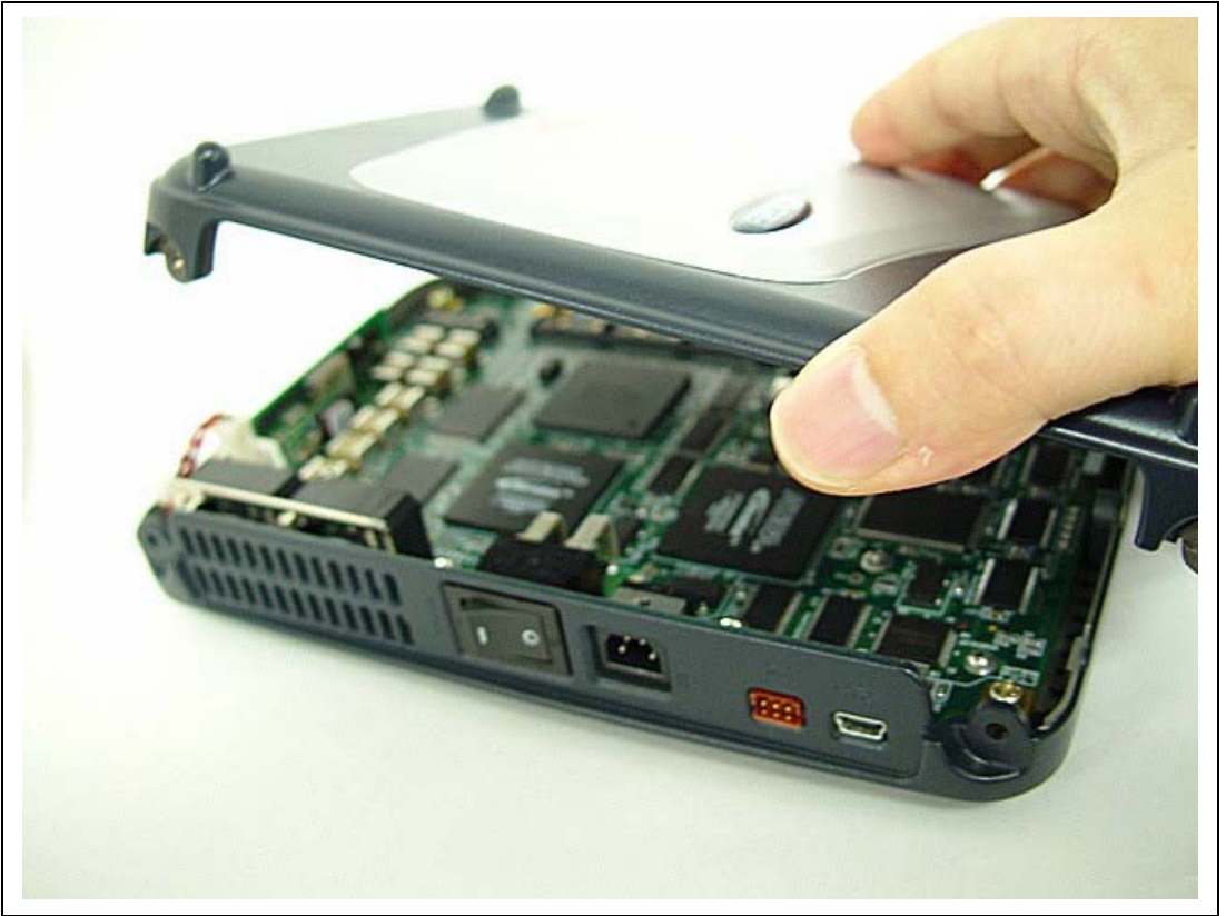
Figure 2.9 Removing the Main Unit Case
