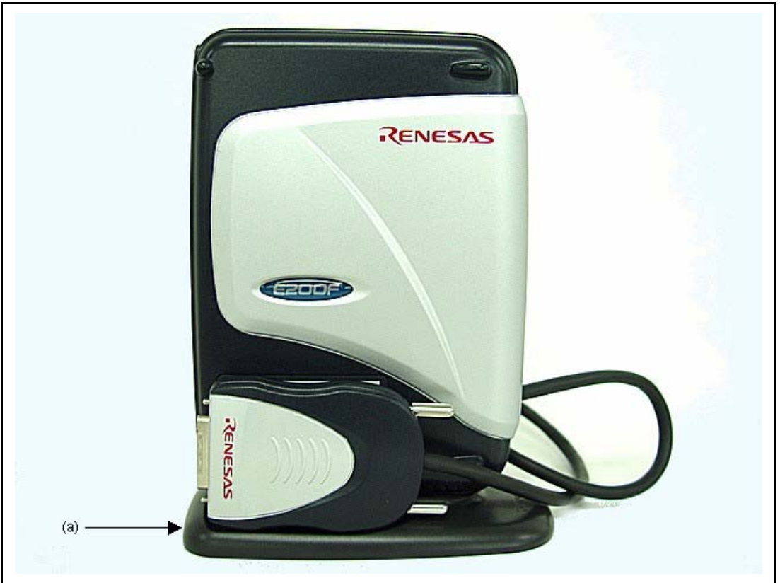
Figure 1.13 Storing the Probe Head (R0E0200F0EMU00)
