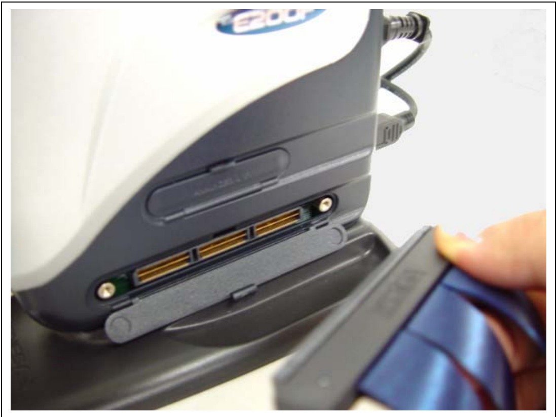
Figure 2.2 Connecting the Trace Cable to E200F
