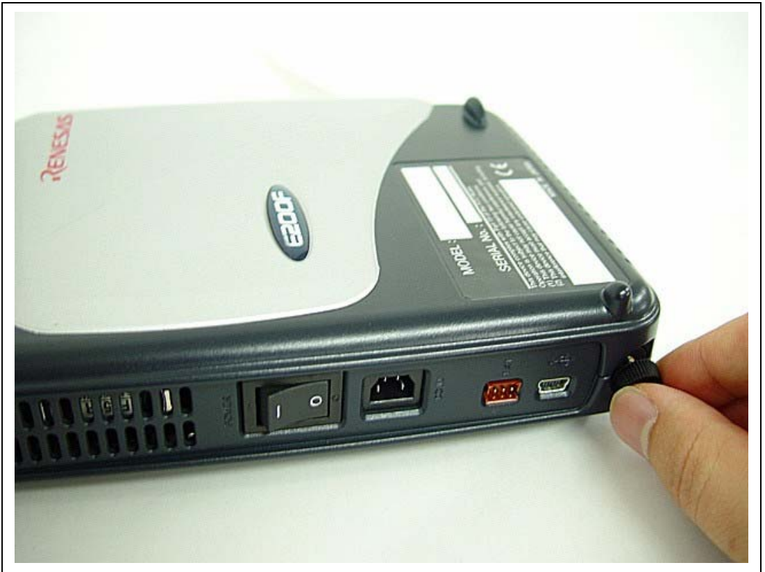
Figure 2.8 Screws for the Main Unit Case
