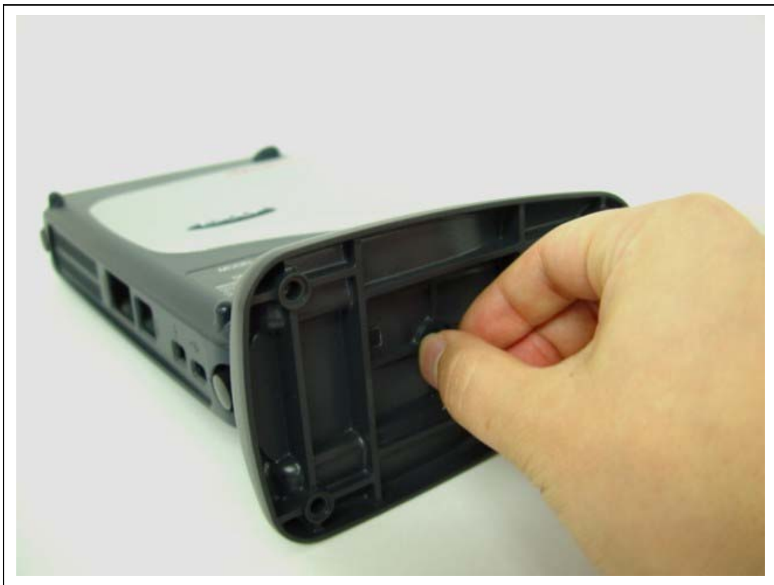
Figure 2.6 Screw for the Base Unit for Placing the Emulator Vertically
